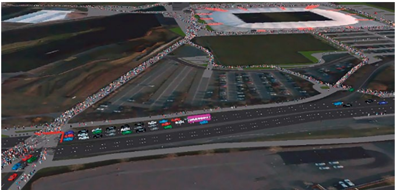
Figure 5: Example of a micro-simulation of arrival at and departure from the public areas of an event [source: ptv AG]
